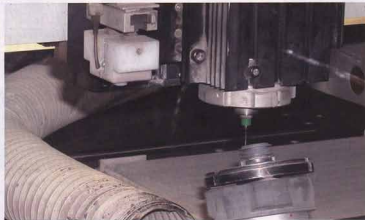
Lava blanks are microdrilled on a high-speed Datron Velociraptor using a fourth and fifth axis at Hypertherm's Hanover, NH, plant. The blanks are machined into plasma-cutter swirl rings.
