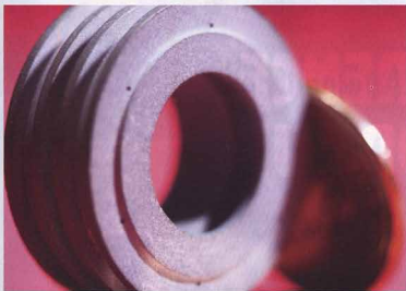
A finished Hypertherm cutter swirl ring with 0.011" (0.28-mm) holes microdrilled in abrasive lava.
