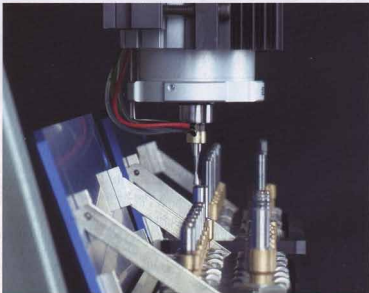
Datron's Automatic Tool Management performs regular tool checks automatically after every 10–20 parts worth of code based on a macro.
